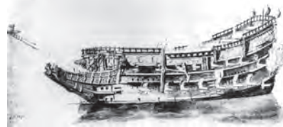
The 41-gun English ship Constant Reformation , she found refuge in Holland in 1648. She was burned in 1649. The presence of an artillery piece at the level of the fore end of the main channel at the third battery shows that this level is not a quarterdeck, but a true deck. The shorter quarterdeck occupies the fourth level. Drawing by Vandevelde the Elder from 1648. - Greenwich National Maritime Museum - Musée de la Marine - pic 91 549
