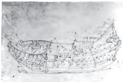
Unidentified Dutch ship. The length of the head indicates that she was built at the beginning of the 1650's. This ship has four levels above the second battery. It is likely that they consist in a quarterdeck and a poop deck, plus two additional levels. In fact it is a three-decker with a quarterdeck, a poop deck, and a half poop deck. Drawing by Vandevelde the Younger of 1656. - Greenwich National Maritime Museum
