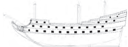
56-gun three-decker pierced for 12 gunports at the lower battery whose line were drawn following the dimensions of the vessel la Royale built in 1661 ( National Archives - Navy - Series B2 - 3 rd Register, folios 33 to 46). Length overall is 133 ft. 4 in. Width of gunports at the lower battery is +/- 32in. Distance between gunports is 7 ft. 9 1/2 in. Depth-in-hold is 12 ft. First battery: 22 18-pounders Second battery: 20 12-pounders Third battery: 10 8-pounders Quarterdeck: 4 4-pounders 1661 (National Archives - Navy - Series B1 - 5 th Register).
