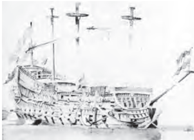
The Bredersde was a 59-gun Dutch vessel of 1646. She was sunk in 1658. At midship of the third deck can be seen a structure that connects the fore and aft parts as on the The Love . Note that this third level that ends forward of the mainmast cannot be a quarterdeck, this type of deck usually ending between the mizzen and the mainmast. Drawing by Vandevelde the Elder probably from 1658.
