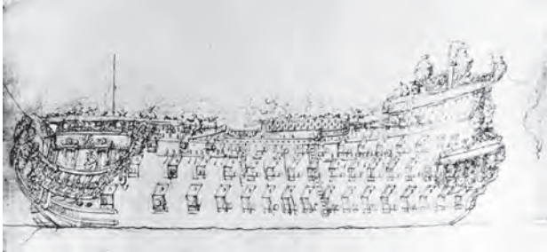
A 100-gun ship, the REINE , built in 1668 at Brest by Laurent Hubac. The REINE was pierced for 16 gunports at the lower battery. Its 100 guns were distributed over three decks, the forecastle and the quarterdeck. The later part topped by an unarmoured poop deck. Drawing from 1673 by Vandevelde the Elder. - Greenwich National Maritime Museum - pic 91 594
