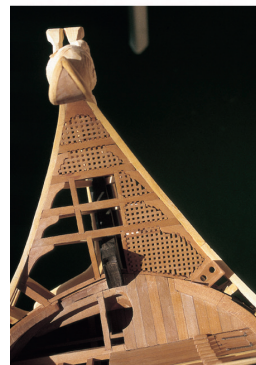
◀ Fitting the rear of the lion's head to the rails is shown in these two views, and also the assembly of the two faces of the scroll to a point. ▶
