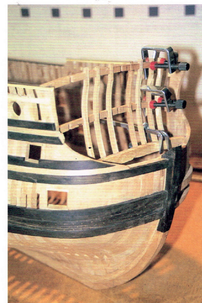
▲ Preparation of the beakhead bulkhead. Note the three beams onto which fit the beakhead bulkhead stanchions.
